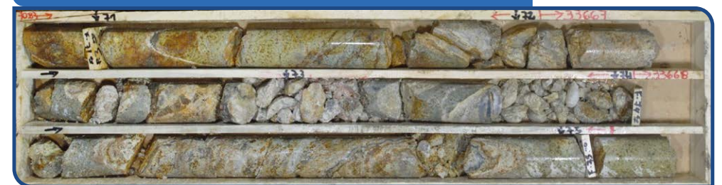
CODD-162: Malvina prospect 7.2m at 14.5gpt AuEq (2.3gpt Au, 854gpt Ag)
